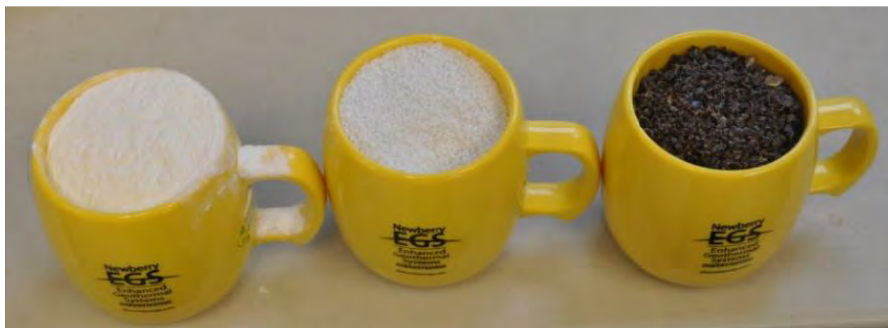
Figure 2-32. TZIM of varying particle size distribution used during Newberry stimulation.
