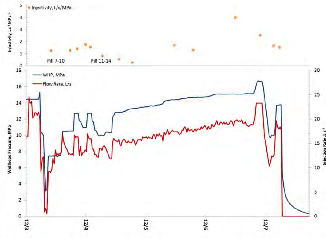
Figure 3-13. Second TZIM injection and Stage 3 stimulation: pressure (blue), injection rate (red) and calculated injectivity (orange).
