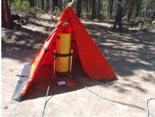
Figure 4-3. Absolute gravity gravimeter survey site preceding stimulation.
