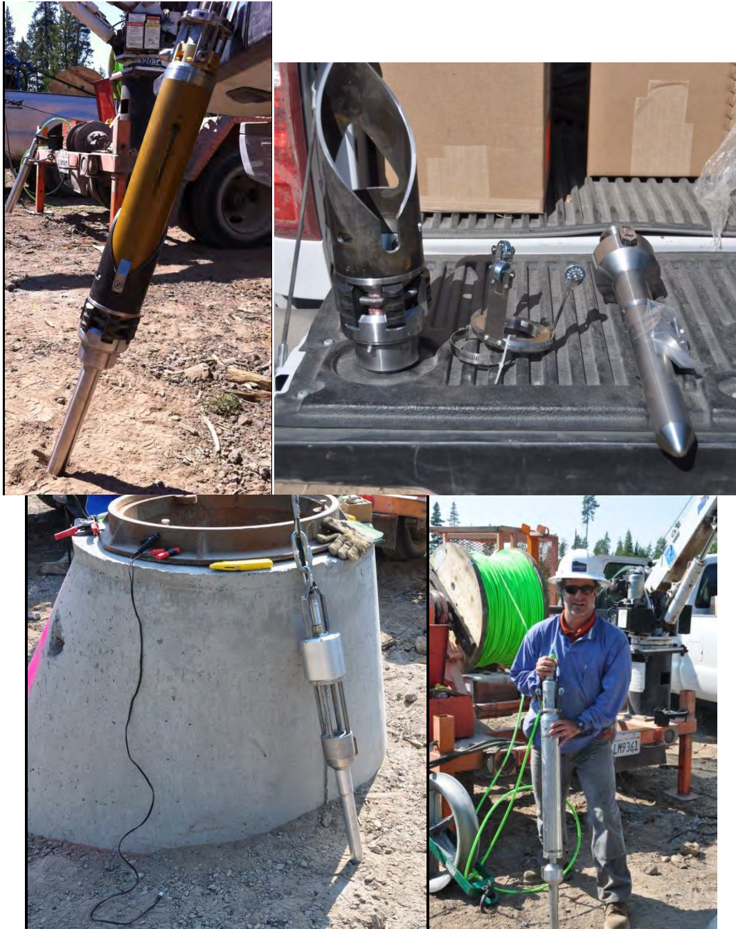
Figure 2-11. Geophone hole-lock installation equipment. Top left: installation tool (a down-hole impact wrench) with hole-lock mounted. Top right: Hole-lock, stabilizer and geophone adapter. Bottom left: Gyroscope for orienting hole-lock. Bottom right: Geophone on data cable (green) ready to install.
